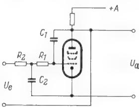
$$f_0 = \frac{1}{2\pi\sqrt{C_1 \cdot R_1 \cdot C_2 \cdot R_2}}$$
